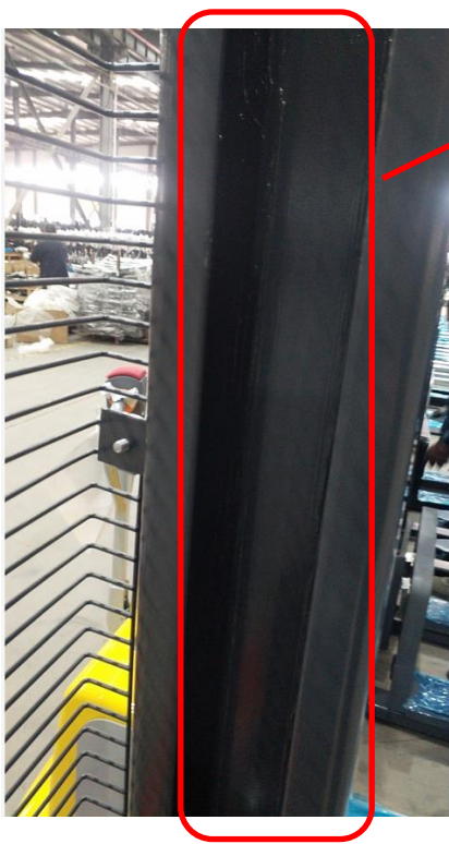
Sliding way in the mast
