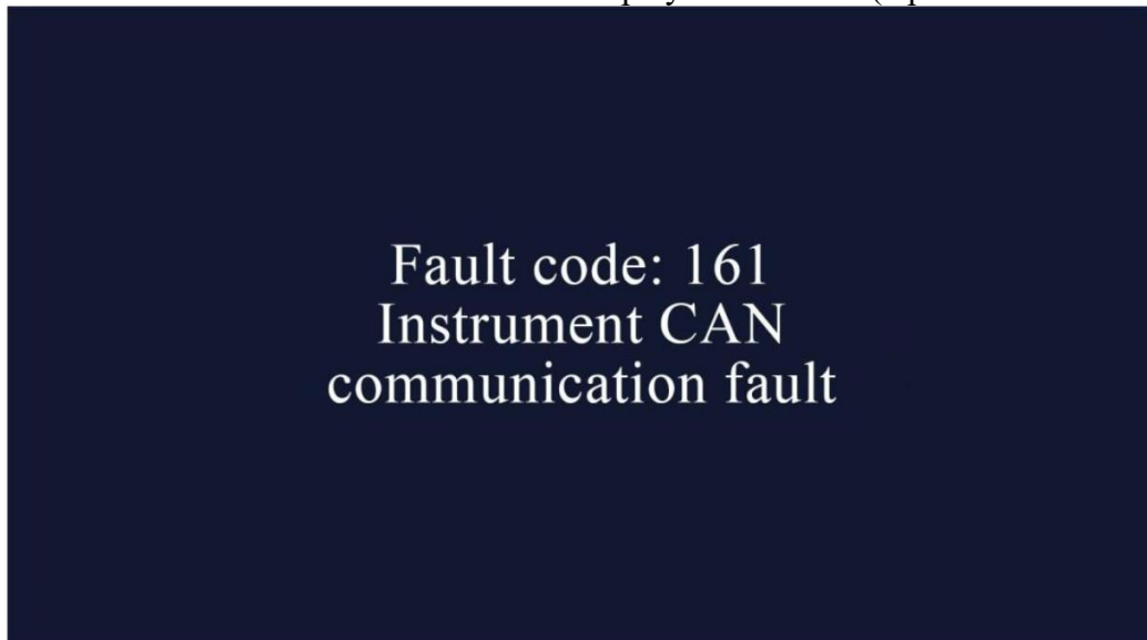
Fig. 4-6 Instrument Interface-Fault Display
