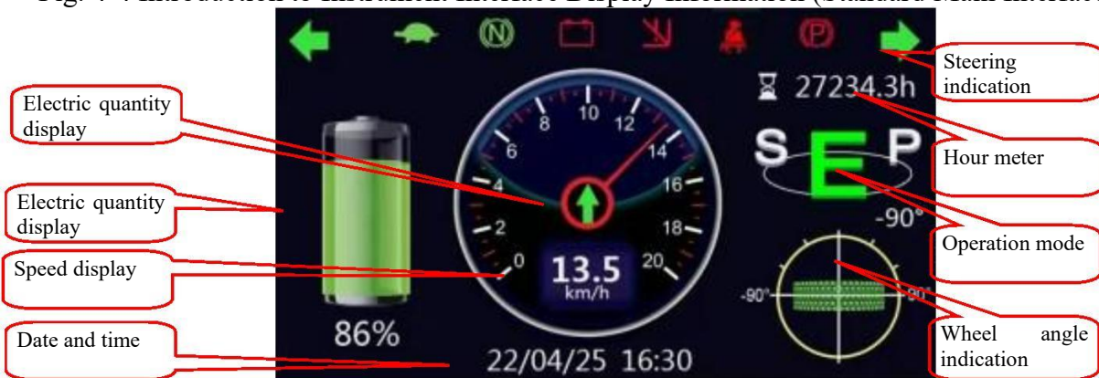
Fig. 4-5 Introduction to Instrument Interface Display Information (Optional Main Interface)
