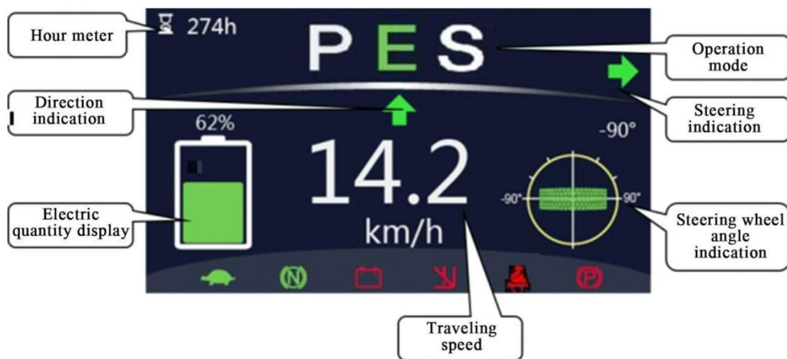
Fig. 4-8 Introduction to Instrument Interface Display Information
