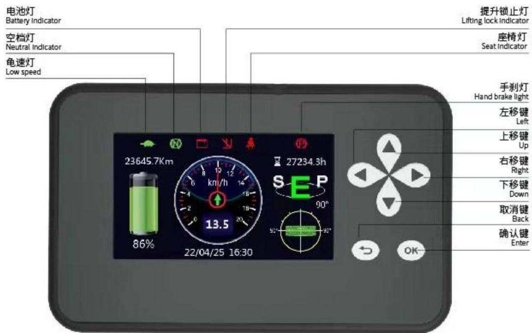
Fig. 4-3 Jiachen Intelligent Instrument Panel (with Jiachen Electronic Control)
