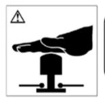
When the forklift is in a variety of emergency situations, the emergency stop button should be pressed immediately.
