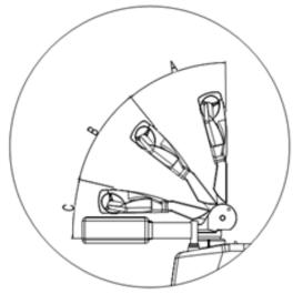
The rudder handle is divided into three sections A, B and C in the vertical plane, and the two zones A and C are the braking zones.
