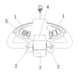
1.Up/Down Button2.Driving Knob4.Horn Button5.Electricity meter
