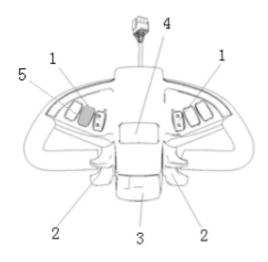
1.Switch for lifting and lowering
