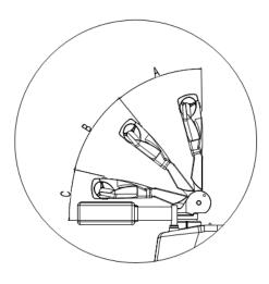
The handle is divided into three sections A, B and C in the vertical plane, and the two zones A and C are the braking zones.
