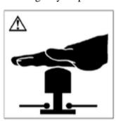
When the forklift is in a variety of emergency situations, the emergency stop button should be pressed immediately.
