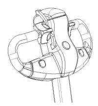
Press the operating handle to the driving state, use your thumb to turn the throttle toward the fuselage, and observe the stacker's retreat; otherwise, observe the forward direction of the stacker.
