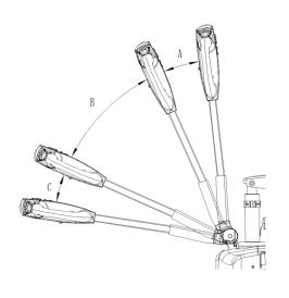
The rudder handle is divided into three sections A, B and C in the vertical plane, and the two zones A and C are the braking zones. When the rudder handle is located in zone A or zone C, the vehicle is in the braking state. If the rudder handle is located in area B, the vehicle is in normal running condition.
